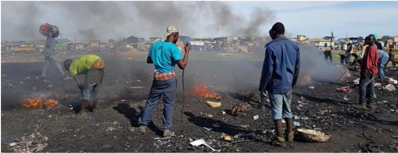
Figure 6.4. Low temperature combustion of polymers associated with wire and printed circuit boards along with other e-waste at Agbogbloshie, Ghana, 2018.
